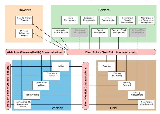
Figure 8.1 Subsystem Diagram
