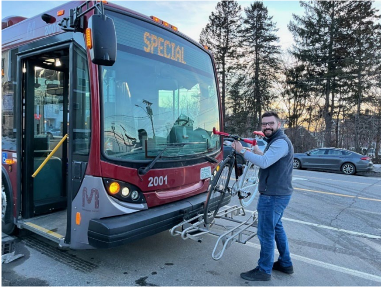
Figure 58: All MTA buses are equipped with bike racks, making it easy for riders to start and end their trip by bike.
